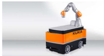
FIGURE 7 – Robot collaboratif mobile KMRiiwa
